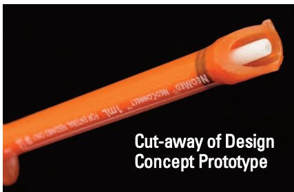
Figure 6. The new NeoMed small volume ENFit syringe design extends the fluid lumen to form a male oriented tip within the female ENFit connector (colored white for visualization purposes only). The white portion inserts inside the internal lumen of an ENFit feeding tube connector, allowing the ENFit syringe to function similarly to oral syringes.
