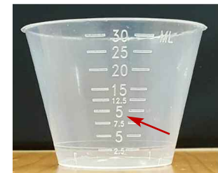
Figure 1. Cup has 5 mL marking where 10 mL marking belongs.
